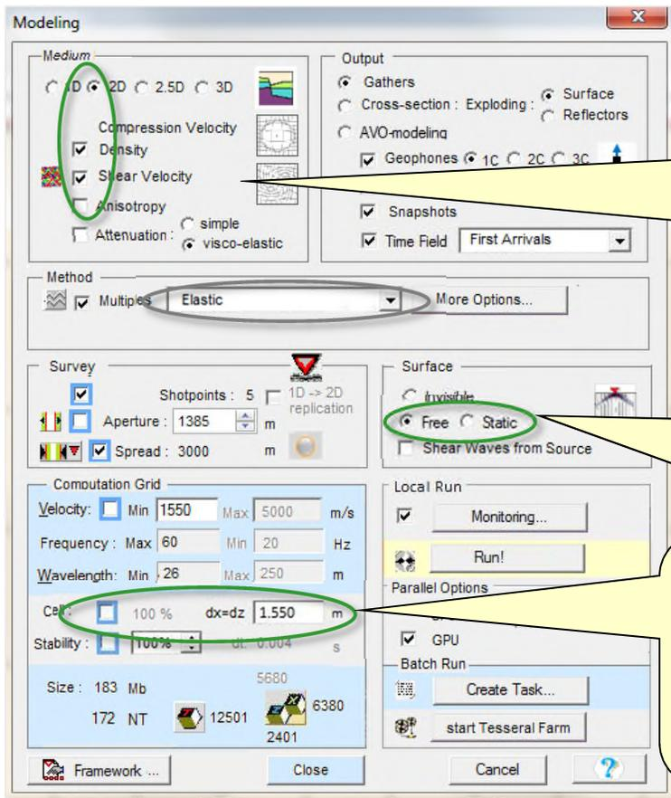
Selecting of used in modeling medium case (2D) and properties automatically determines type of used wave equation approximation.
