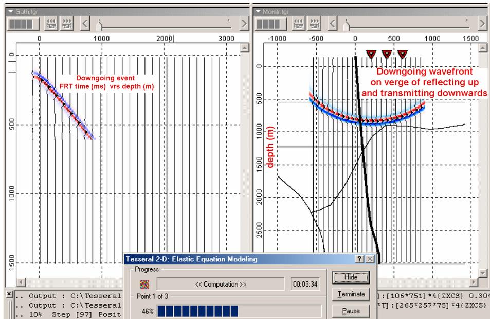
As the computation continues, we see that the downgoing wavefield is about to reflect from the “reef-like” structure.
