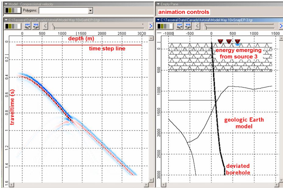
We see a time step line on the VSP data. This is used during the animation process. The animation process will replay the generation of the wavefronts in a movie fashion. The time step line shows how the VSP data is being generated as the wavefronts in the movie propagate. The animation icons in the two panes look like
