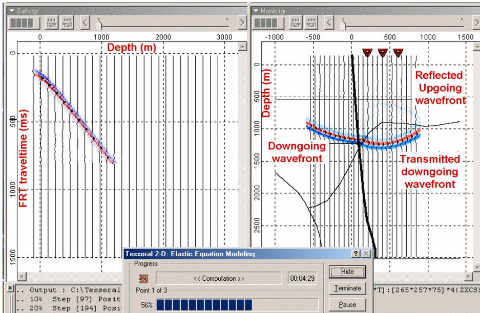
Note the reflected upgoing wavefront. The amplitude of the downgoing event can be 100 times larger than the upgoing events ... so the upgoing VSP event is difficult to see on the VSP (on the left) without proper scaling.
