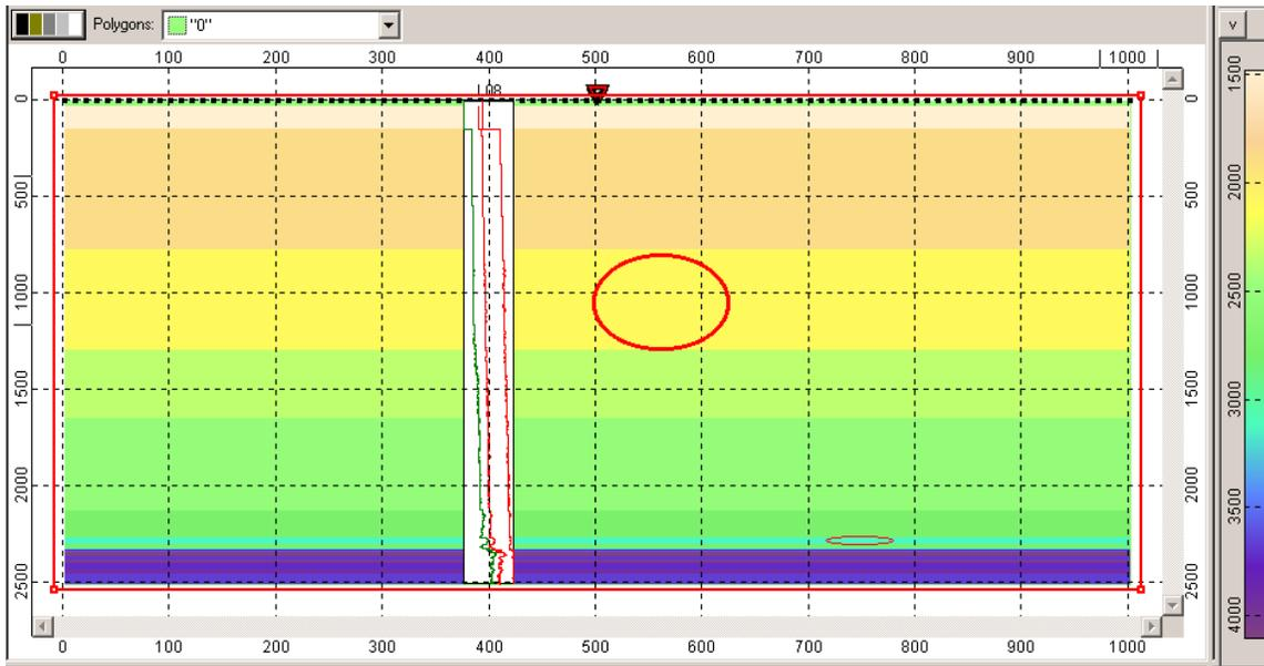
Here we see the model ... some of the layers are thick and some are thin. The thin layers are nearer to the bottom of the borehole ..
