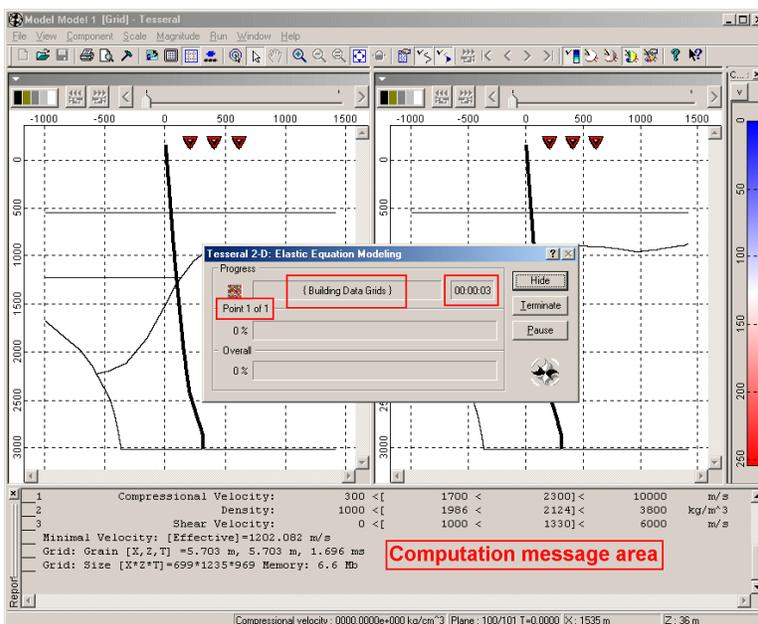
Once the grid is built, the computation begins for source number 1. Note the propagation of the modeled wavefront and the downgoing events recorded in the well.
