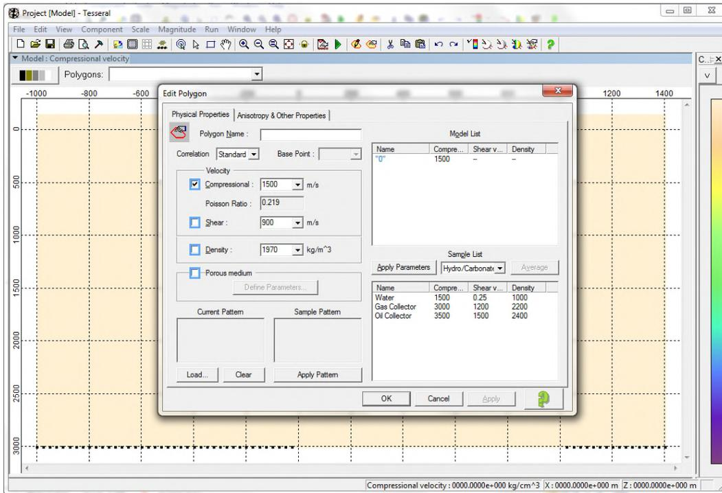
In the menu, we can start by defining the *P*-wave velocity. The *S*-wave (*shear*) velocity and density will assume default values (the defaults will be used when the *blue boxes*  are unchecked).
