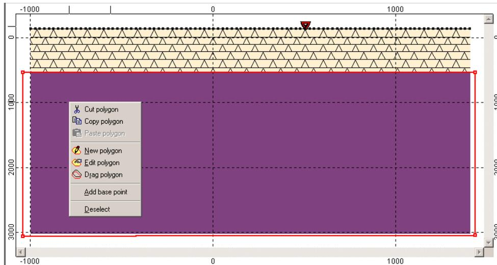
*Polygon 3* will start from the left side of the model and truncate against *Polygon 4*. How do we do this? We first input *Polygon 3*. Then we construct *Polygon 4* so that it cuts through *Polygon 3*.
