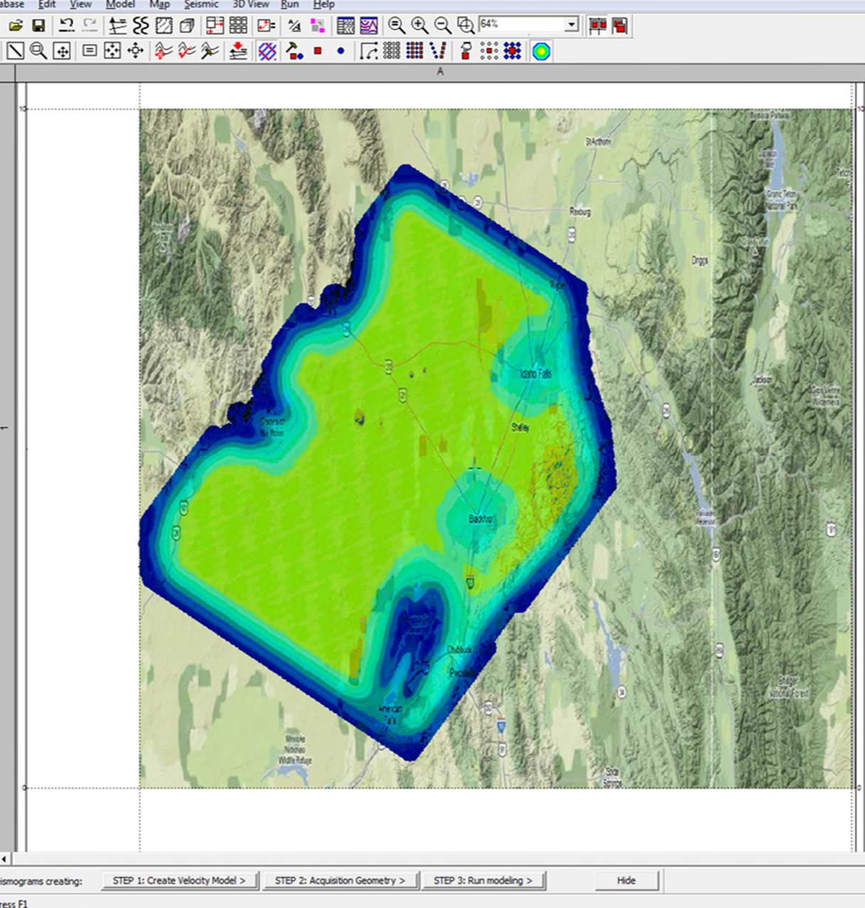
Calculate Theoretical 3D Survey Fold for picked bin size .
