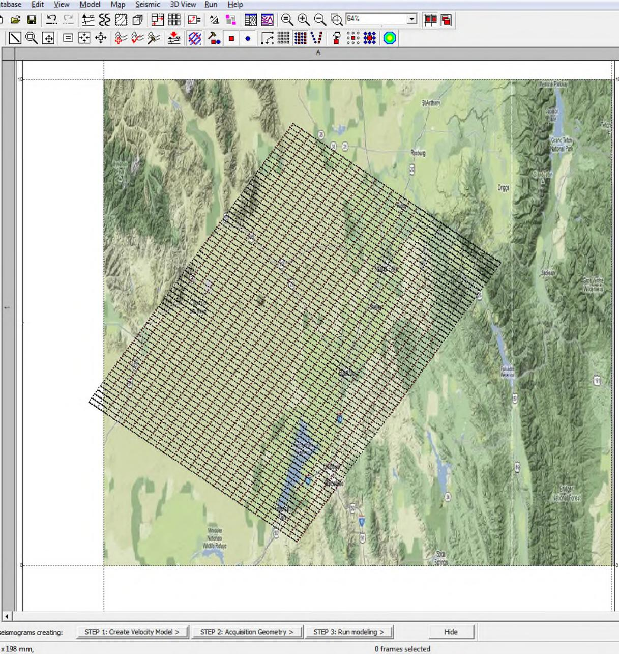
Using Topographic plan it is possible to overlay it with desired 3D Survey Planning Map, correct number, direction and distance between In-Lines and Cross-lines; edit positions of Shot and Receiver Stations.
