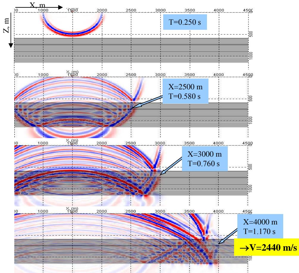
Determining of effective velocity by synthetic shotgather, based on the thin-layered model
