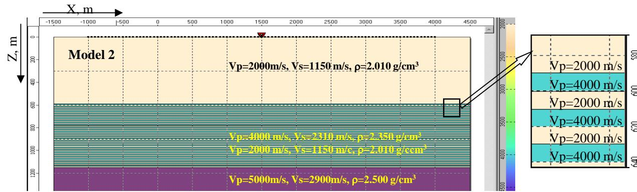
Determining of velocity  $\alpha_{\parallel}$  for acoustic model 2 by the head wave propagation
