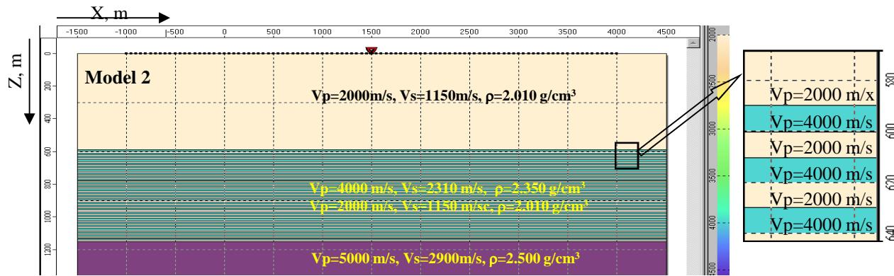
Determining of velocity  $\alpha_{\parallel}$  for elastic model 2 by front of the head wave propagation fixed in time moments:
