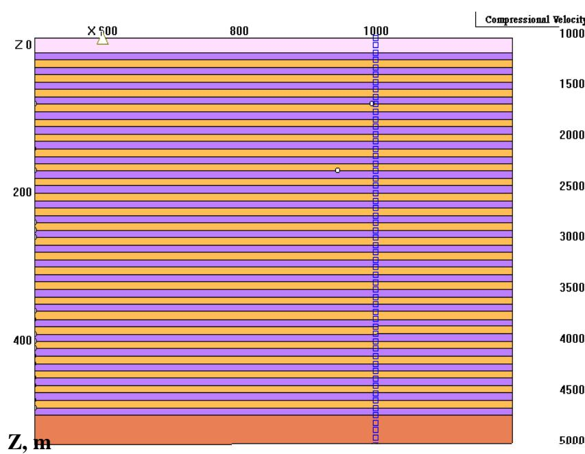
Quasi-anisotropy effect in condition of the thin-layered model can be demonstrated for VSP data at studying of polarized properties of the downgoing compressional wave by its Z- and X- components
