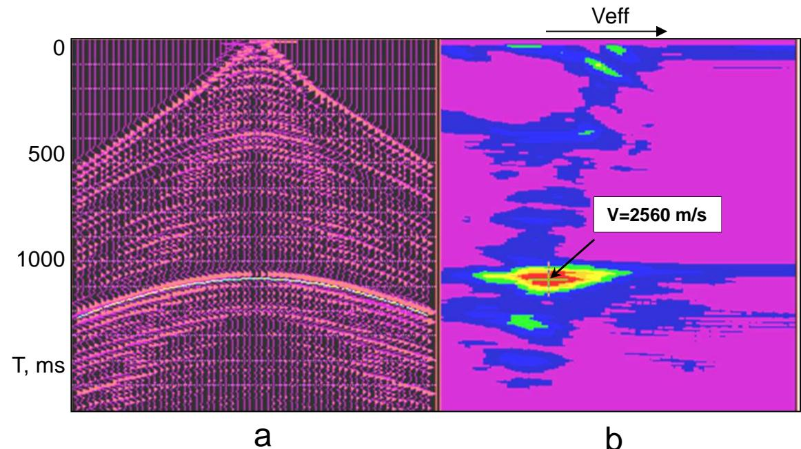
Determining of effective velocity by synthetic shotgather, based on the thick-layered model
