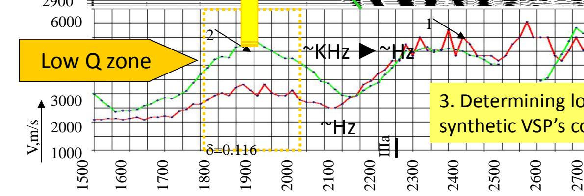
Velocity analysis of the wave propagation for real VSP in comparison with SL  $\rightarrow$  synthetic VSP velocities determined in the well S-2 on the Black Sea shelf : a – thin-layered velocity model by the well SL; b – model shotgather; c – graphics of interval velocities, determined on the base 100 m,  $V_{\text{VSP}}$  (1 – ) and  $V_{\text{SL} \rightarrow \text{VSP}}$  (2 – ).
