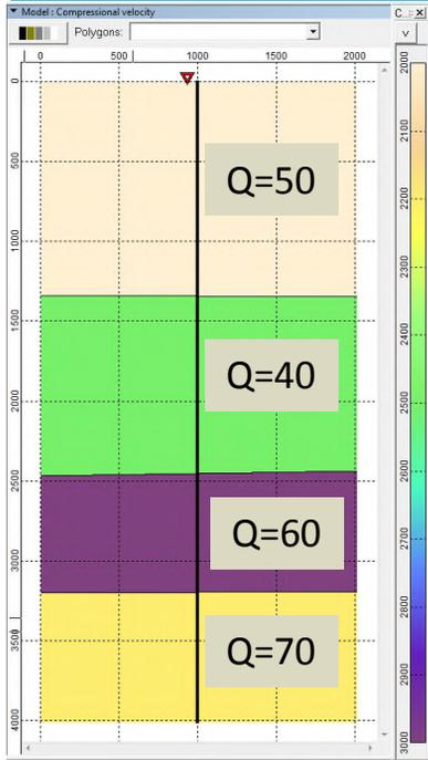
Source model with absorption *Q-factor values close to the average ones for sediment rocks*
