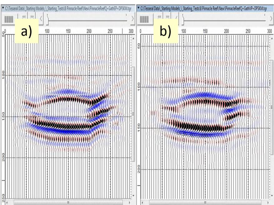
**Left (a)** – synthetic PSDM cross-section produced from **Elastic** gathers;
