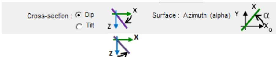
Anisotropy modeling mode allows entering Thomsen's parameters: Epsilon, Delta, Gamma (between -0.2 and 0.2) tilt angle Phi (between -90° and 90°) and azimuth (between -180° and 180°, 3D case extension). Those values can be entered for any polygons of the model (not necessarily for all)
