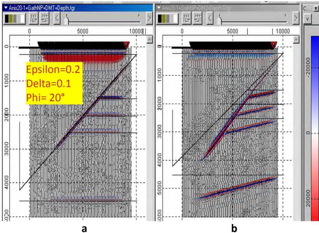
Comparison of migrated cross-sections with source model (shown on background); when anisotropy is taken into account (a) and when anisotropy is not taken into account (b).
