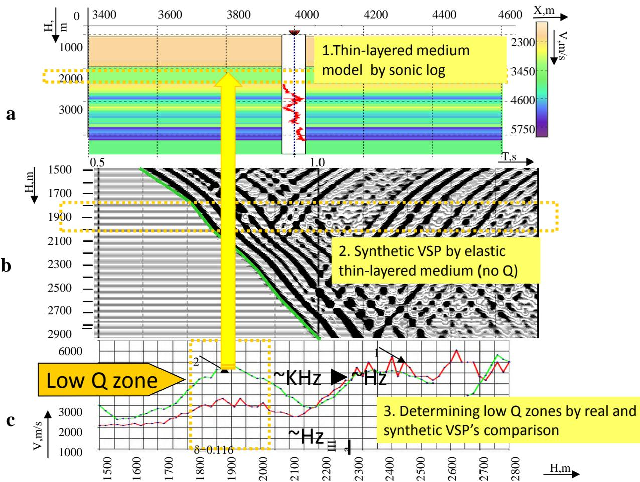
Velocity analysis of the wave propagation for real VSP in comparison with SL → synthetic VSP velocities determined in the well S-2 on the Black Sea shelf : a – thin-layered velocity model by the well SL; b – model shotgather; c – graphics of interval velocities, determined on the base 100 m,  $V_{VSP}$  (1- —) and  $V_{SL \rightarrow VSP}$  (2- —).
