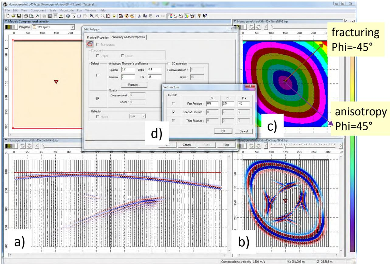
Shotgather (a), Snapshot (b) and Time field (c) of first arrivals in anisotropic fractured medium for model with inclined anisotropy and fracturing axes. It can be seen that strong anisotropy and fracturing (d) can considerably distort propagating S-wave field (b).
