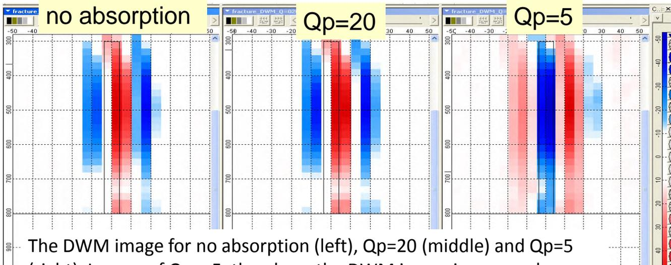
The DWM image for no absorption (left),  $Q_p=20$  (middle) and  $Q_p=5$  (right). In case of  $Q_p = 5$ , the phase the DWM image is reversed.
