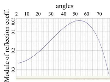
**Figure 6** The AVO-curve obtained by the base boundary by a priori geological data
