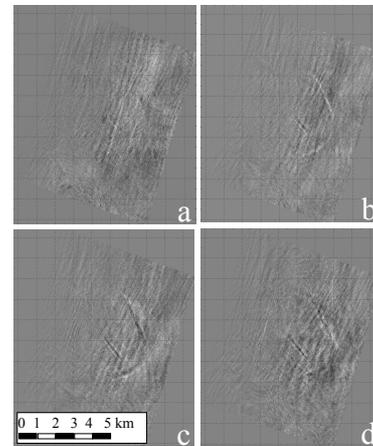
**Figure 4** The stratigraphic slices of the partial DWM cubes obtained above the target interval boundary with apertures relative to the source points in the intervals
