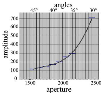
**Figure 5** The AVO-curve obtained by partial cubes within the lineament shown by the red arrow in the Figure 3.
