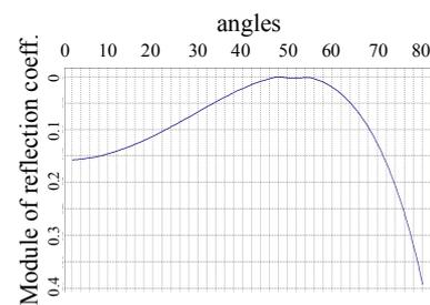
**Figure 7** The prognostic AVO-curve on the target sub-vertical boundary
