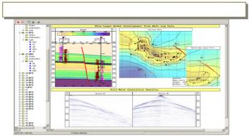
Tesseral Pro enables the creation of **thin-layered models capable of high precision and modeling feasibility**. Along with well log data, the user can enter additional data such as: well's coordinates and inclinometry, stratigraphic arrangements, fault information, horizon maps etc.
